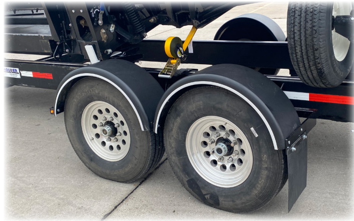
60291 - 235/85R LRG STEEL BELTED RADIAL TIRE ON ALUMINUM WHEEL 801822 - BOLT-ON POLY REAR FENDERS, REMOVABLE
