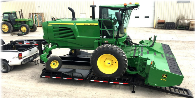
LOADING A 16' SP WINDROWER ON A SW30XD
