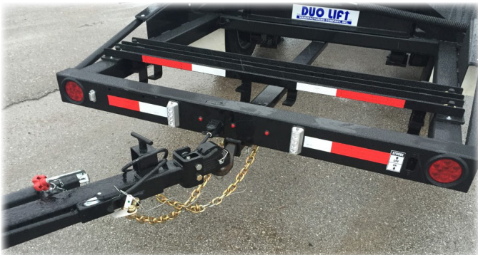
REAR HITCH IS INCLUDED ON THE SW25HD, SW30HD AND SW30XHD MODELS
