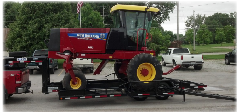
WINDROWERS CAN BE LOADED WITHOUT A HEADER
