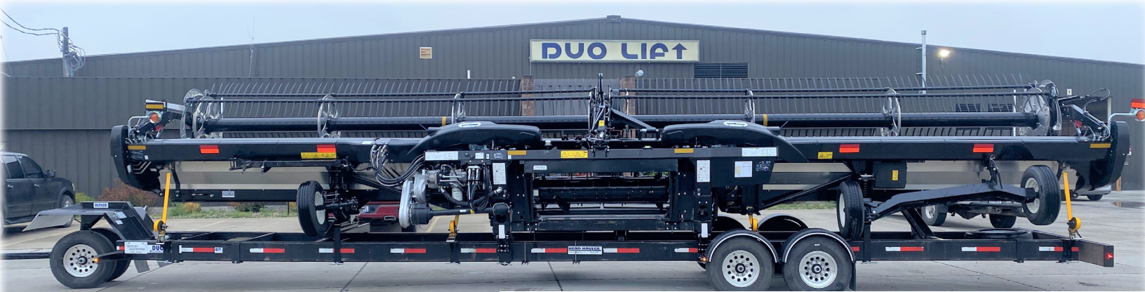
MODEL SHOWN: DLT42D D.O.T. COMPLIANT HEAD HAULER, SHOWN WITH MACDON FD240 FLEX DRAPER
