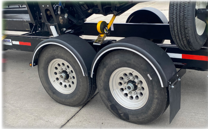
60291 - 235/85R LRG STEEL BELTED RADIAL TIRE ON ALUMINUM WHEEL BOLT-ON POLY REAR FENDERS STANDARD ON D.O.T. FRONT-STEERS
