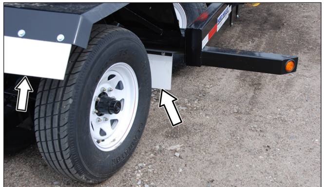
Front and Rear Mud Flaps on Front Axle.
