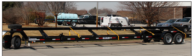
DLT42D and DLT47D Equipped with Four Header Bar Supports.
