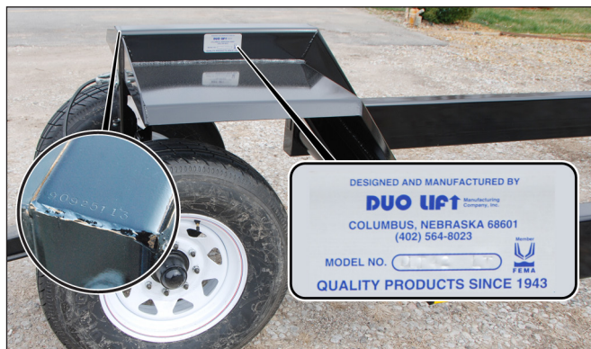
Model number plate on standard DL, DLT, and DLTLT model trailers. Serial number is stamped on top of frame.
