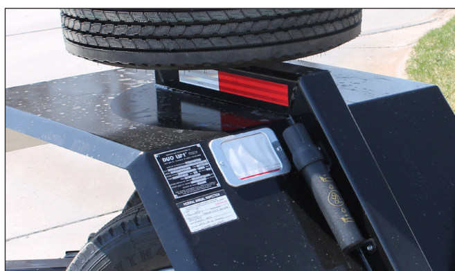
VIN, model, and serial number plate on DLTD model trailer.
