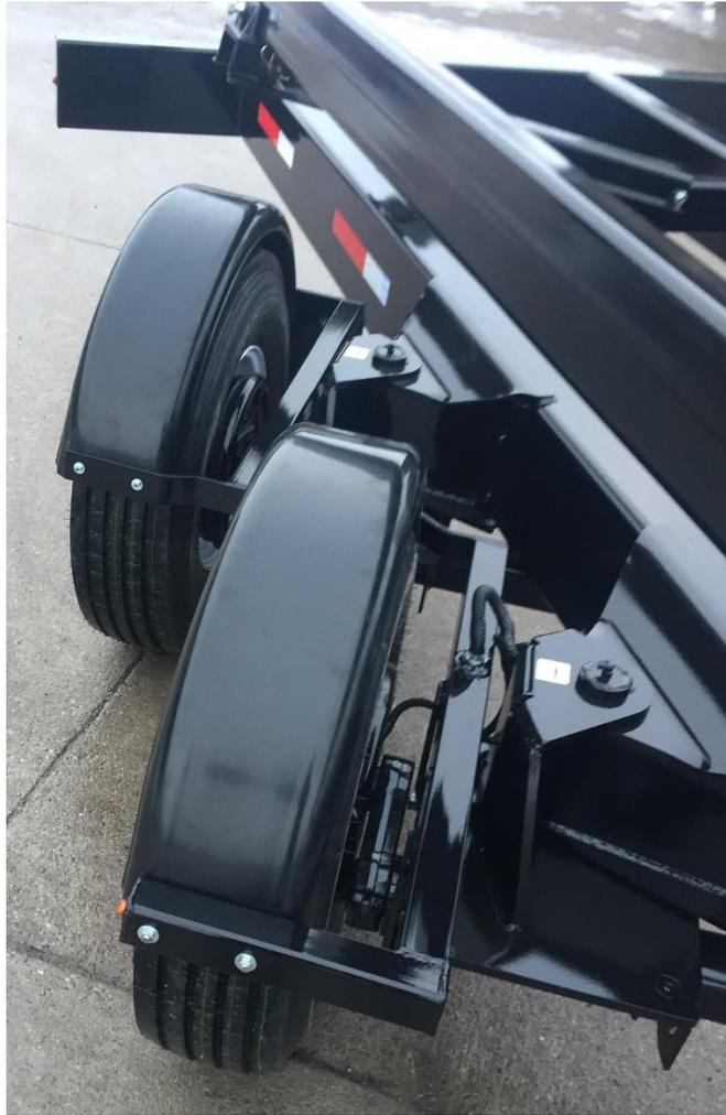
**All Wheel Steering of Front Dolly Wheels and Rear Tandem Axles with Electric Brakes, Fenders and Torsion Suspension**
