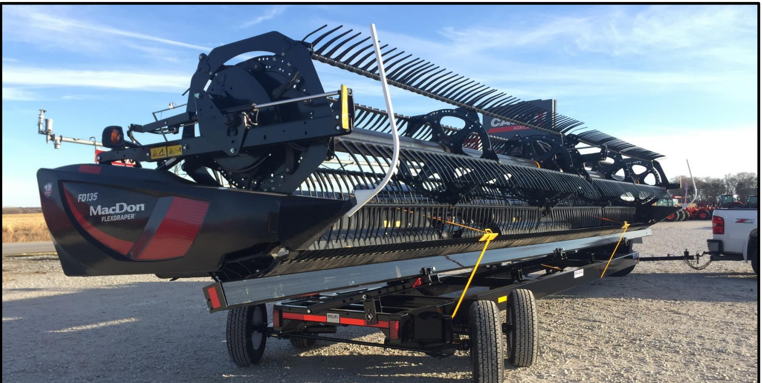
AST37LT Shown with 35' Flex Draper - Trailer in Full, "All Steer Position"
