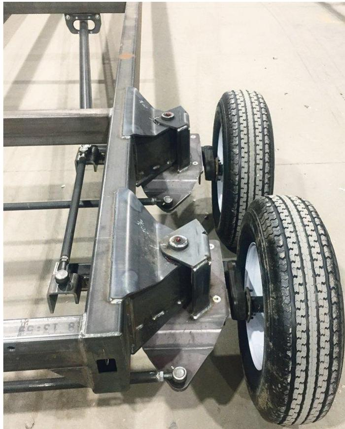
**The long tie rod makes the rear tires steer in the opposite direction of the front tires, allowing the rear of the trailer to swing out and around for a tighter turn radius. | Duo Lift Photo**
