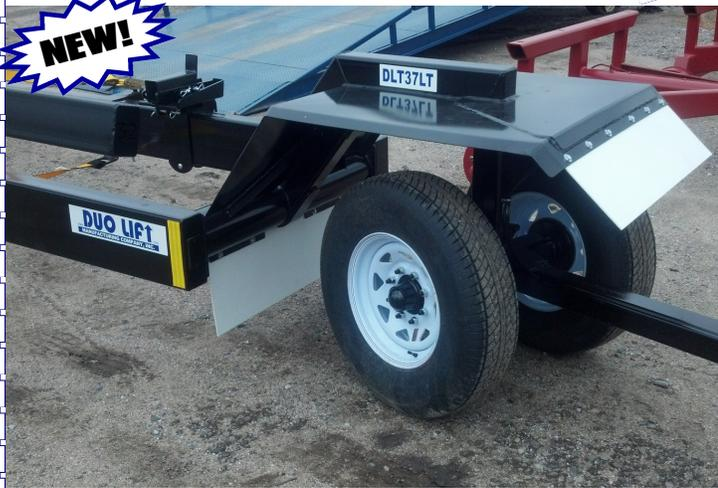
P/N 801003 Extended Coverage Front Steel Fender and Splash Guards Option
