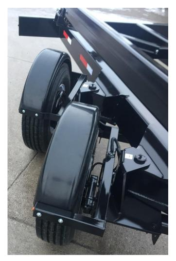
All Wheel Steering of Front Dolly Wheels and Rear Tandem Axles with Electric Brakes, Fenders and Torsion Suspension
