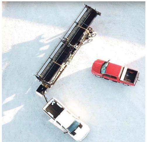
The ability to move a big header in tight yards and around other machinery makes the Duo Lift trailer unique. | Duo Lift video still
