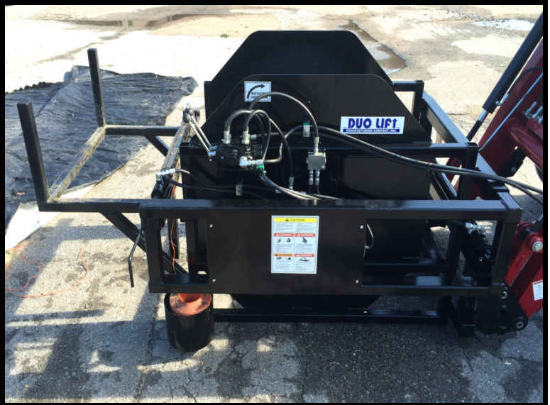
Two Lever Control Valve, Twin Bag Release Cylinders, Twine Ball Canister and Manual Twine Wrapper
