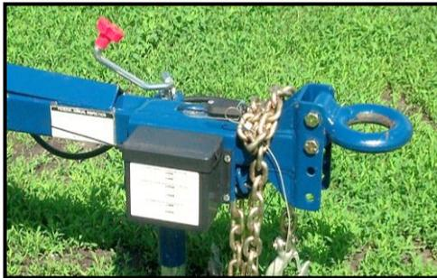
Optional Equipment: Heavy Duty Tongue with Adjustable Height Pintle Hitch, Safety Tow Chains, Lights, Electric Brakes and Tongue Jack.
