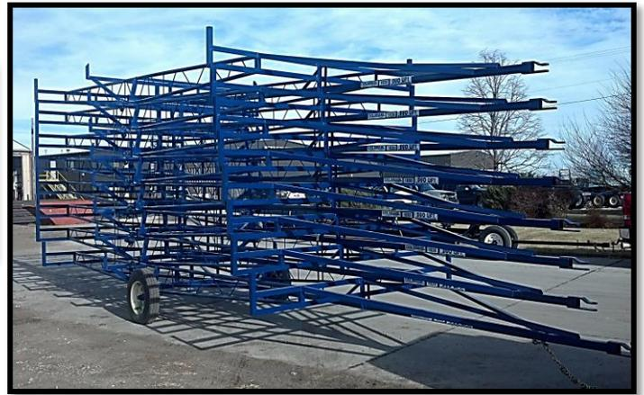
Pipe Trailers can be Stacked in Stacks of 2 to 10 Trailers Depending on the Trailer Size for Efficient Trailer Delivery.
