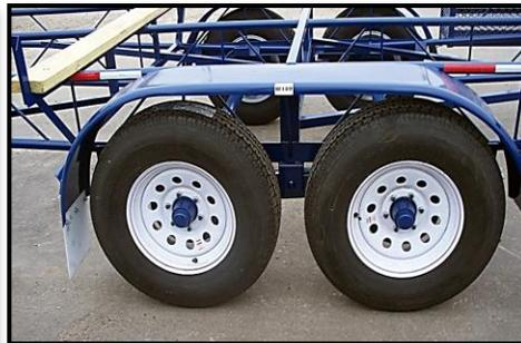
Optional Equipment: 6000 Lb. Tandem Axles, 16" Highway Speed Radial Tires on 6 Bolt White Spoke Wheels, Fenders with Splash Guards, D.O.T. Conspicuity Tape and Treated Wood on Cross Members.
