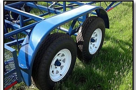
Optional Equipment: 3500 Lb. Tandem Axles, 15" Highway Speed Radial Tires on 5 Bolt White Spoke Wheels and Fenders.
